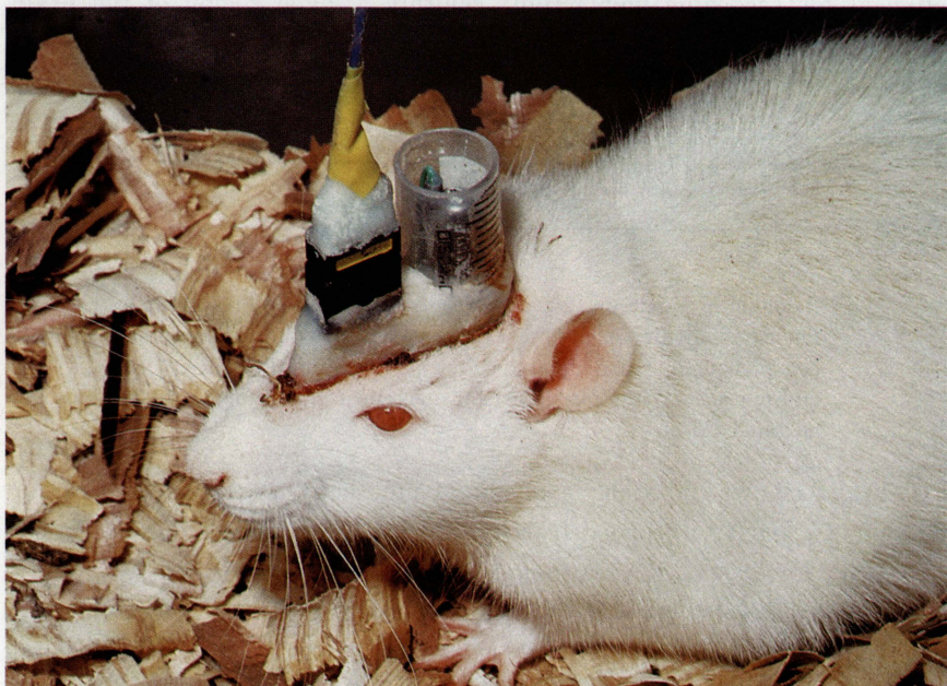
Fig. 2 Photograph of a rat with the microdrive assembly mounted ready for use.
